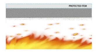
When exposed to high temperature, the coating starts to react between 86°C and 100°C, and the chemical process causes the coating to expand. An insulating char is formed and evaporation on the surface of the char has a cooling effect.
