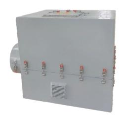
Prefabricated modular type - Daken Epoxy Coating Shell (DEC) Passive Fire Protection Systems can be designed as a fully removable system that can be installed at site. The retrofit design is compact and quick to install using quick-release toggle fasteners. The system is self-supporting and can be adjusted easily at site to allow for tubing and cables to exit.
