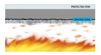
During the early stage of the fire, the char on the surface of the coating increases, reflecting 80-90% of the heat away from the protected item.
