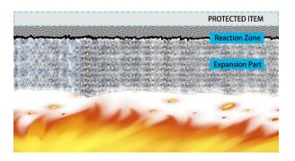
As the fire exposure continues, the heat will penetrate the outer layer, allowing the inner layer of the epoxy coating to chemically react. Once the material has fully reacted and a char has formed, the material will prevent temperature rise over a given duration.
